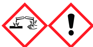
Corrosion Exclamation mark
